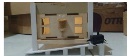
Fig. 3. Miniature prototype of the IoT-enabled smart layer hen coop used in laboratory unit testing
